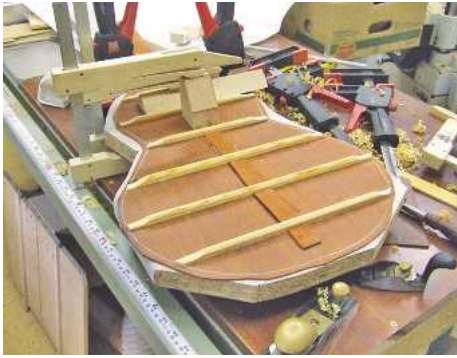
▲ Pic.10 Also, use off-cuts of wood as cauls to cramp the grafts in place
